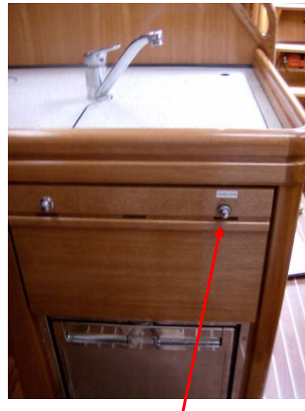
Fridge drain button
