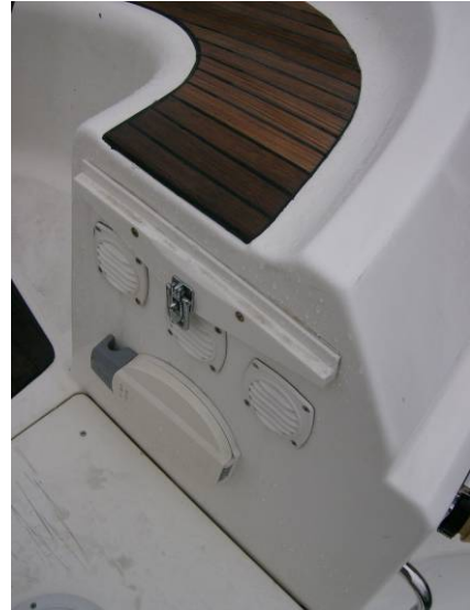
The manual bilge pump is located at the starboard helm
